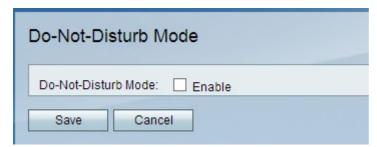
Step 2. In the Do-Not-Disturb Mode field, check the **Enable** check box to turn off the LEDs on the front panel of the device.
