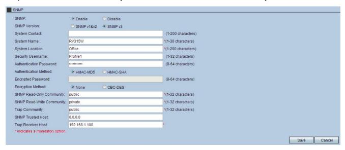
Step 7. (Optional) Enter a username in the Security Username field. This is the username that is used in order to gain access to the SNMP setup.
