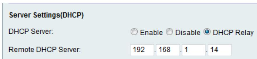
The screenshot shows a configuration window titled "Server Settings(DHCP)". It contains two rows of settings. The first row is "DHCP Server:" with three radio button options: "Enable", "Disable", and "DHCP Relay". The "DHCP Relay" option is selected. The second row is "Remote DHCP Server:" followed by four input fields containing the IP address "192", ".168", ".1", and ".14".
