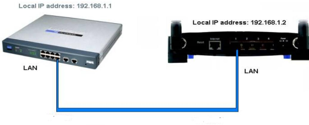
**Note:** If you can access the GUI of both routers from your PC that is plugged in to either of the routers, then your routers are cascaded successfully.
