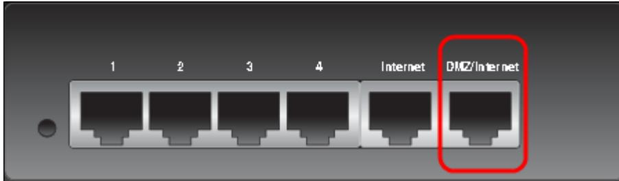
**Note:** To use a secondary ISP, a second IP address is needed from the ISP. The second WAN port or DMZ/Internet port on the router can be configured as a DMZ port or as a secondary ISP port. The default setting for the secondary WAN port is an ISP connection. To change this setting, log in to the web configuration utility and edit the WAN settings.
