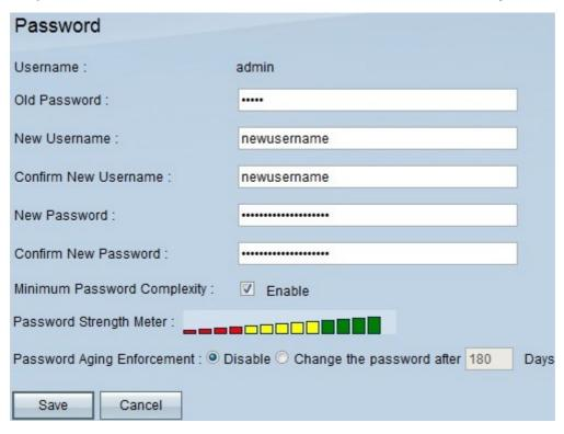
Step 2. Enter the existing password, that you used to initially access the device, into the Old Password field.
