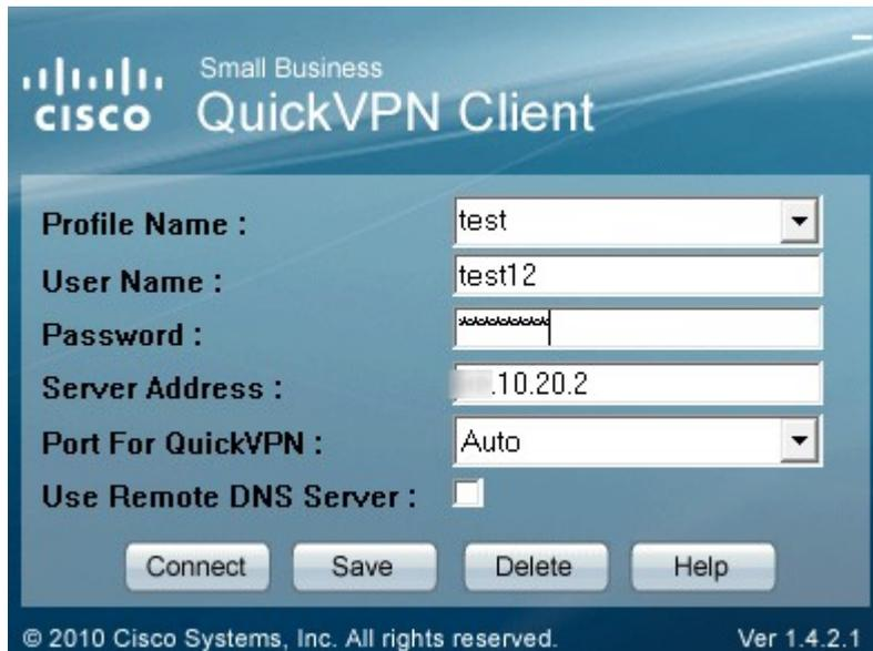
Step 6. Click **Save** button to save the connection settings in a profile with given name test. Click **Connect** for connecting to the WRVS4400N remotely.
