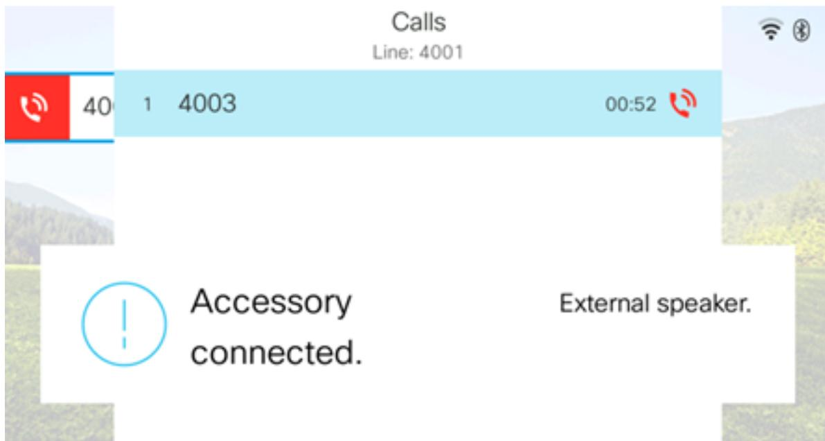
**Note:** In this example, a Plantronics VXI X100 V1.1 headset is plugged into the USB port of the Cisco IP Phone 8861 Multiplatform Phone. The Headset button lit amber and the call is transferred from the external speaker to the headset.
