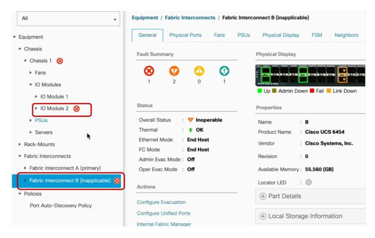
Upon completion, verify that the new firmware version is installed on the subordinate Fabric Interconnect by selecting the **subordinate Fabric Interconnect**, in this case **Fabric Interconnect B** in the **Equipment** section of the navigation pane.
