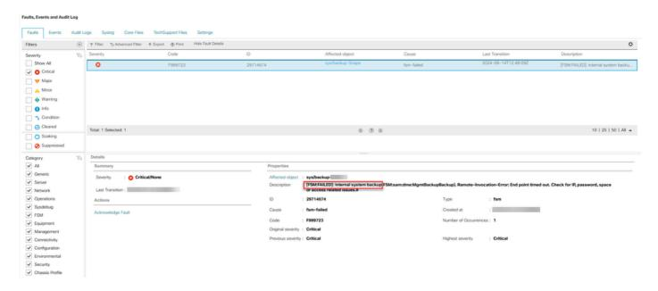
This fault can arise if there is a communication error between the Primary and Secondary Fabric Interconnect.
