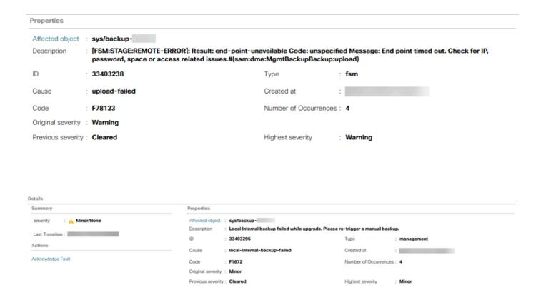
This fault indicates that the UCS Domain was unable to successfully connect and transfer the backup file to the configured destination server.
