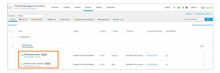
Finally, bring up/reconnect the data interfaces of the FTD2 device.
