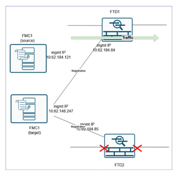
If you have a VPN configuration attached to the FTD2, you have to remove it first before deleting the FTD. In different case, a message similar to this is shown:
