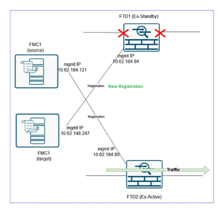
**Step 9. Import the FTD Device configuration object into the FMC2 (target FMC)**
