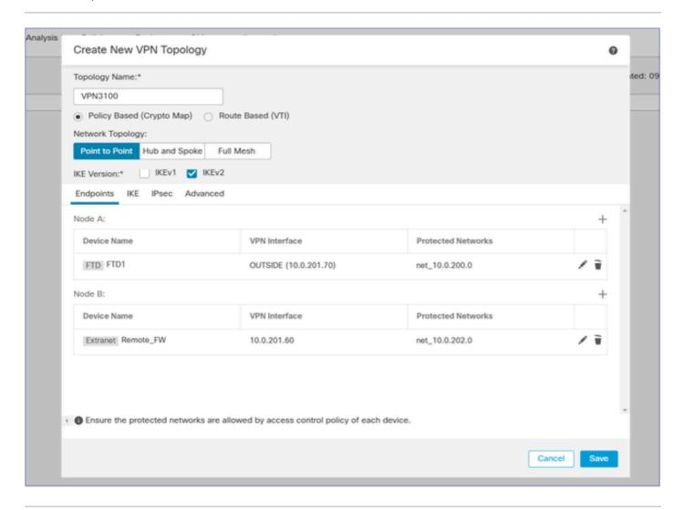
Note: If the FTD that is migrated has S2S VPN peers that are also migrated to the target FMC, you have to configure the VPN after moving all FTDs to the target FMC.
