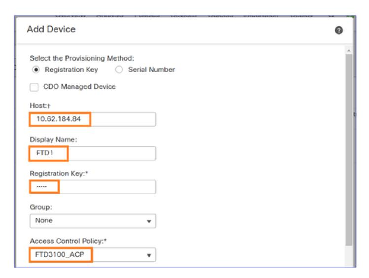
Apply the needed licenses and register the device:
