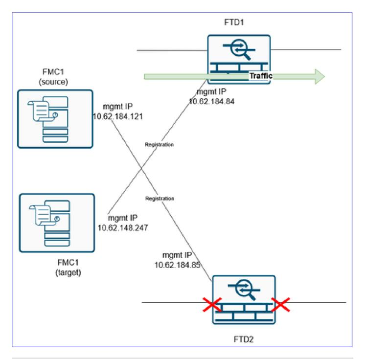
Caution: Arrange a MW to do the cutover. During the cutover you are going to have some traffic interruption until all the traffic is diverted to the FTD1, VPNs are re-established, and so on.
