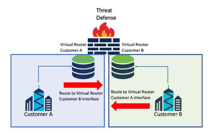
• In each virtual router, configure a static route that points to the destination network with the interface of the other virtual router.
