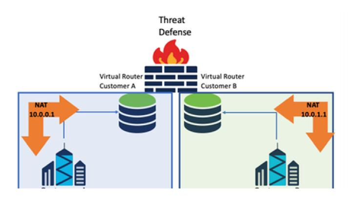
In order to have communication between the 2 networks, configure a twice NAT to override the source IP address and put a fake IP address.
