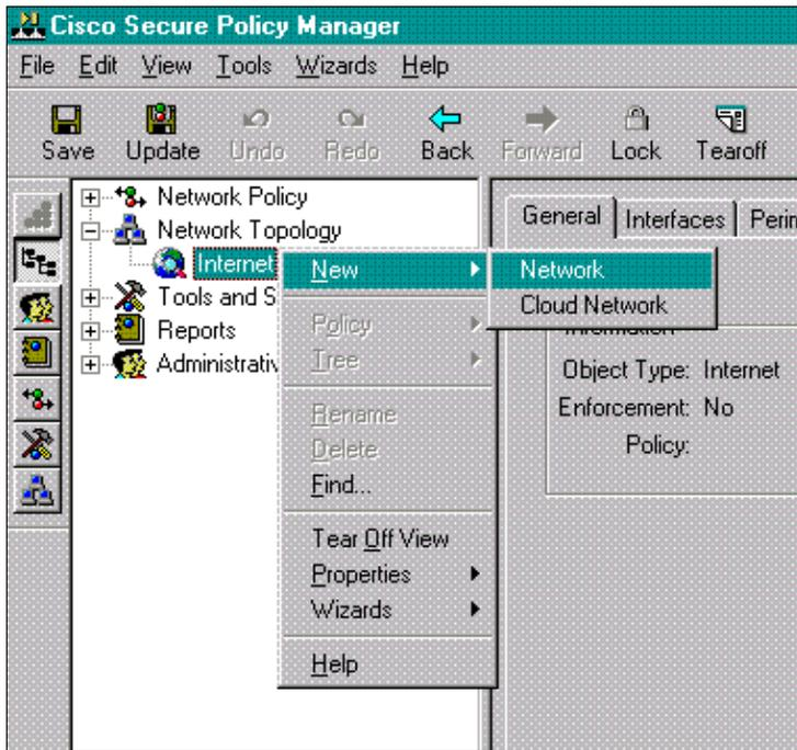
2. On the right hand side of the Network Panel, add the name of the new network, the network address, and the netmask that will be used.
