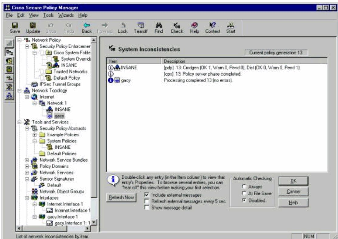
5. Select the Sensor in the network topology and click the Command tab to send the updated configuration to the Sensor.
