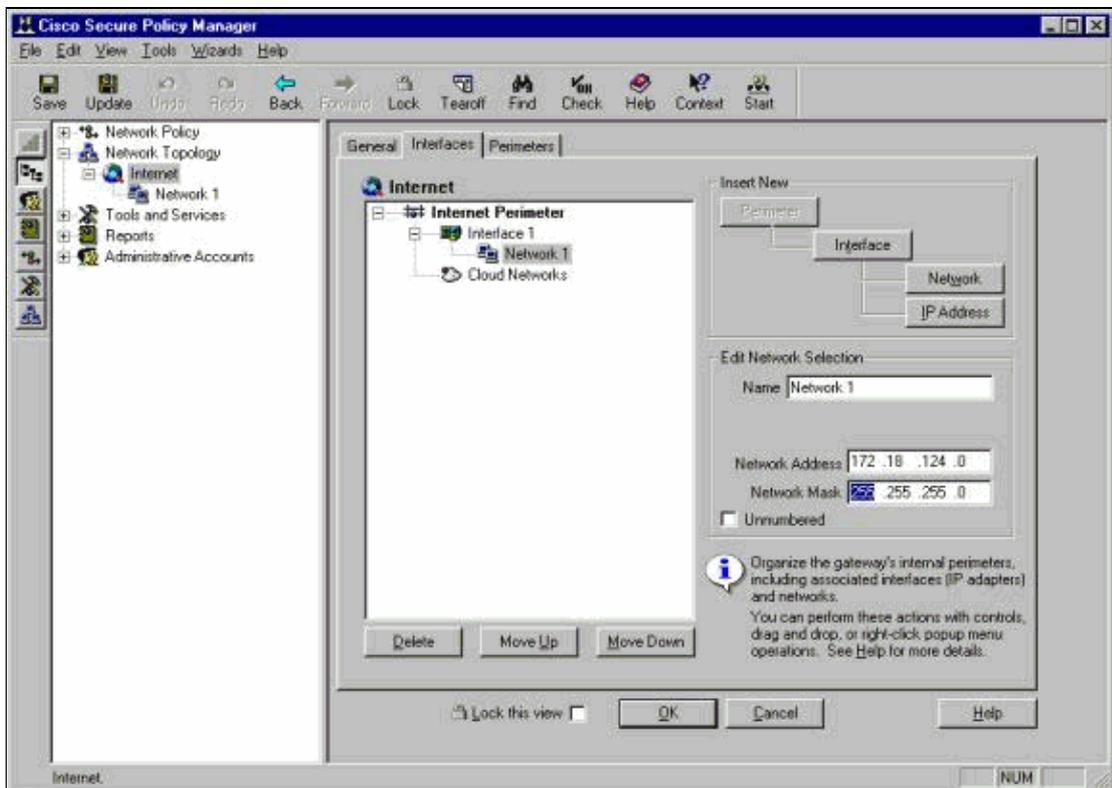
3. Click the **IP Address** button, and enter the IP address for your network that it uses to reach the Internet.
