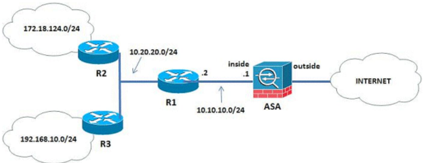
In the network topology that is illustrated, the Cisco ASA inside interface IP address is 10.10.10.1/24. The goal is to configure EIGRP on the Cisco ASA in order to learn routes to the internal networks (10.20.20.0/24, 172.18.124.0/24, and 192.168.10.0/24) dynamically through the adjacent router (R1). R1 learns the routes to remote internal networks through the other two routers (R2 and R3).
