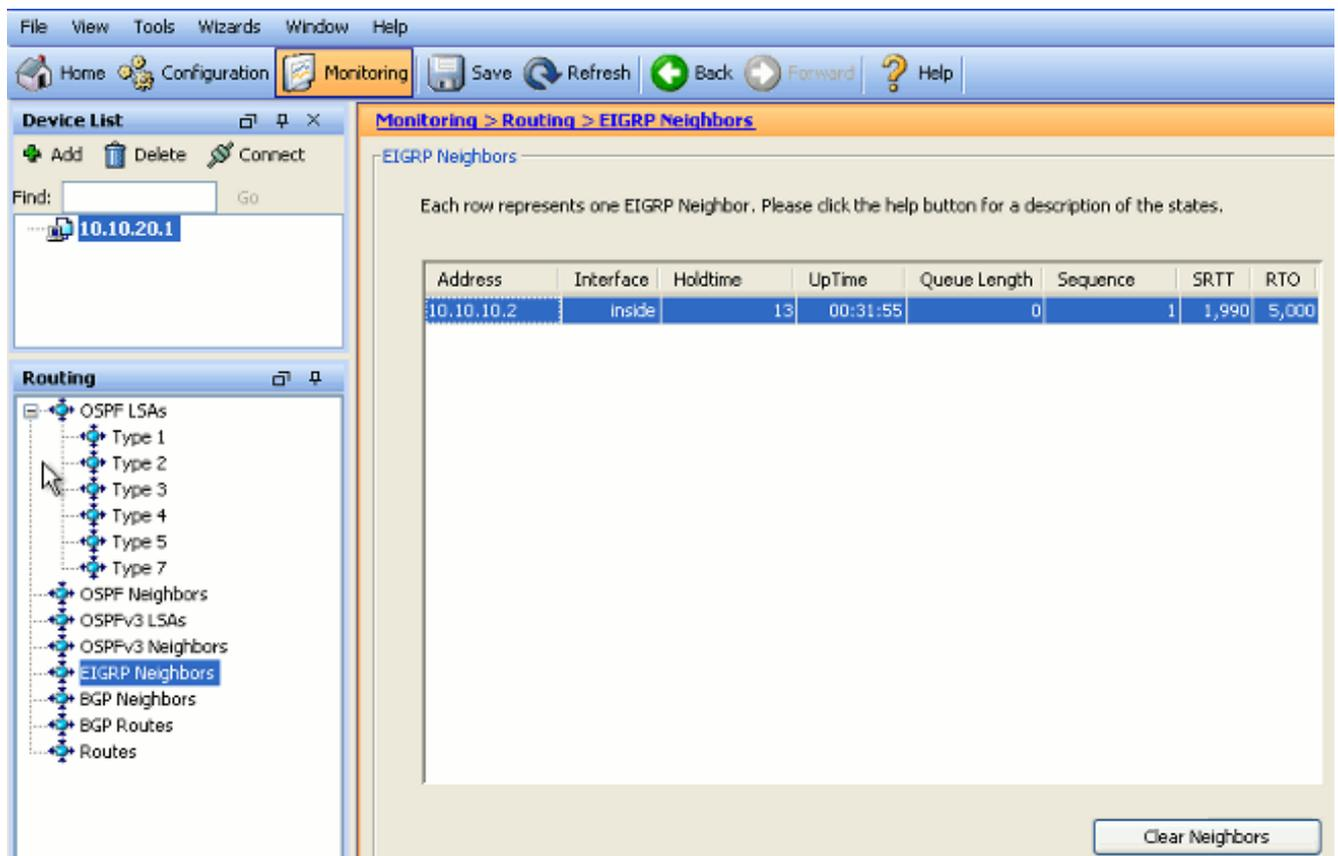
2. Additionally, you can verify the routing table if you navigate to **Monitoring > Routing > Routes**. In this screenshot, you can see that the **192.168.10.0/24**, **172.18.124.0/24**, and **10.20.20.0/24** networks are learned through R1 (10.10.10.2).
