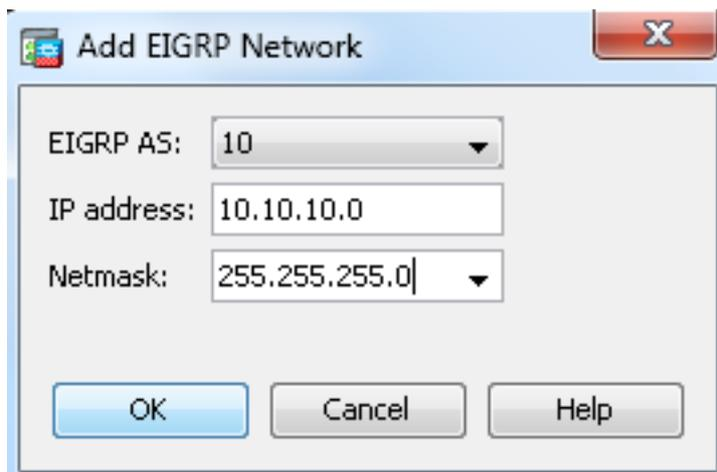
Only interfaces with an IP address that falls within the defined networks participate in the EIGRP routing process. If you have an interface that you do not want to participate in EIGRP routing but that is attached to a network that you want advertised, configure a network entry on the **Setup > Networks** tab that covers the network to which the interface is attached, and then configure that interface as a passive interface so that the interface cannot send or receive EIGRP updates.
