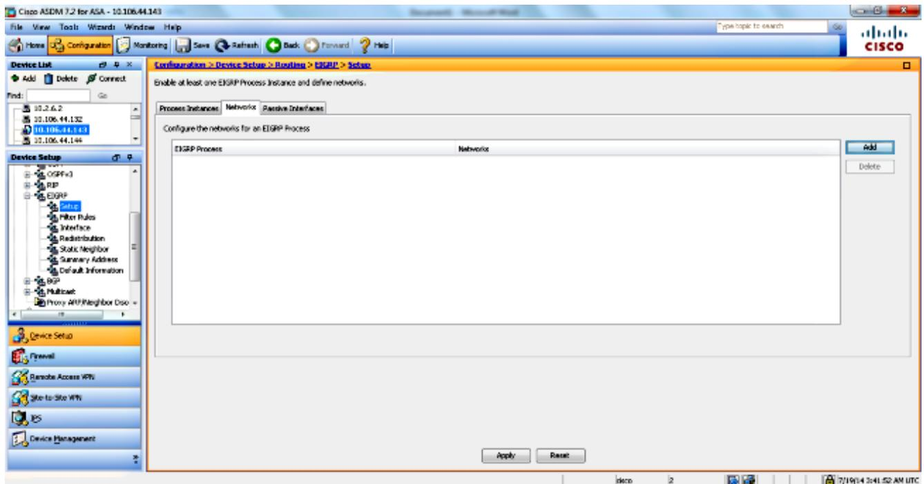
6. This screen appears. In this example, the only network that you add is the inside network (10.10.10.0/24) since EIGRP is enabled only on the inside interface.
