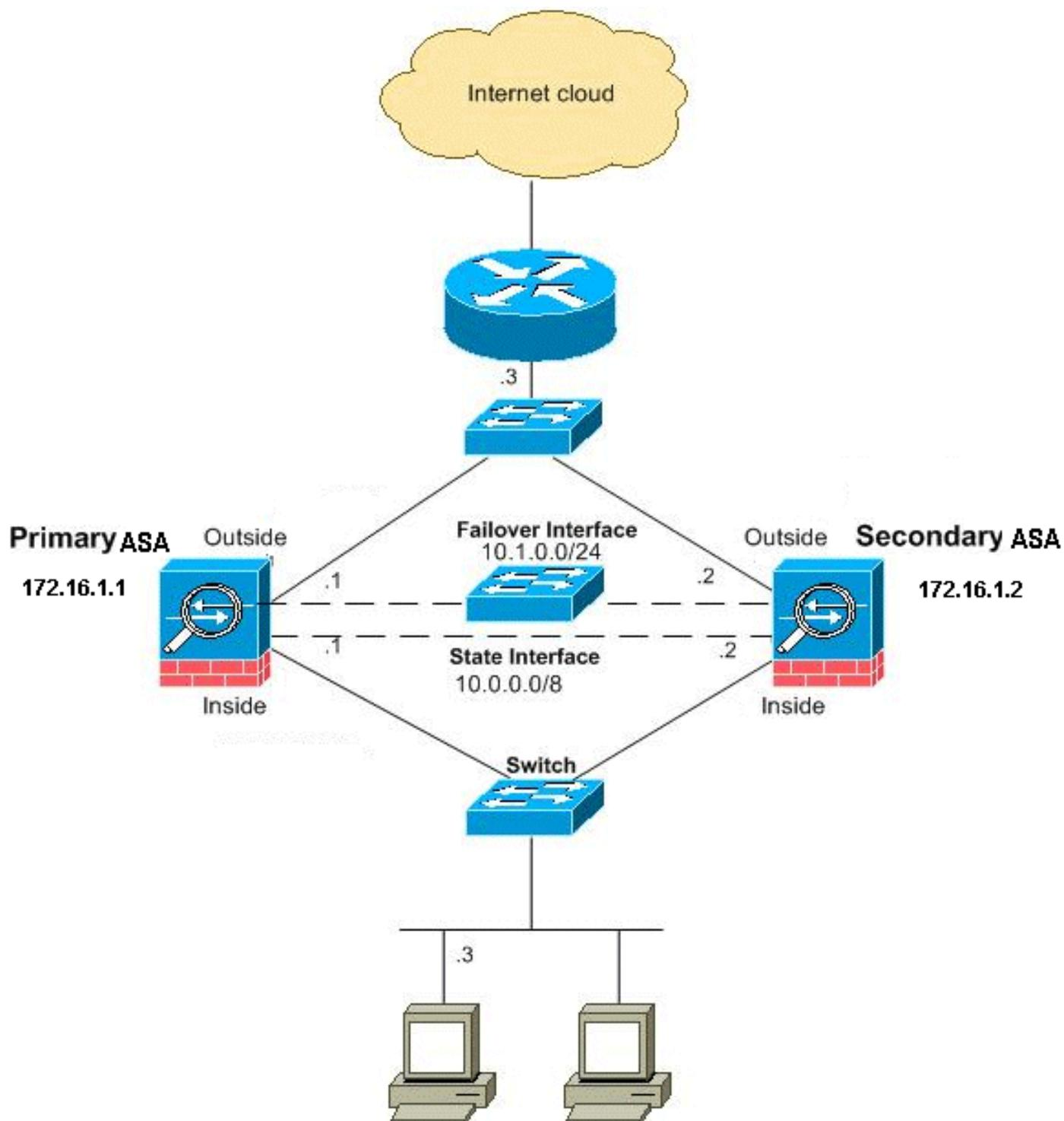
This section describes how to configure Active/Standby Failover in Transparent mode with an Ethernet failover link. When you configure LAN-based failover, you must bootstrap the secondary device to recognize the failover link before the secondary device can obtain the running configuration from the primary device.
