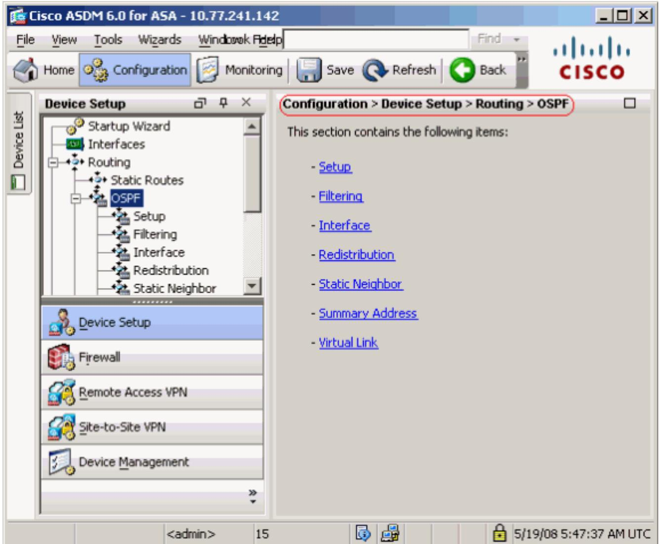
Enable the OSPF routing process on the **Setup > Process Instances** tab, as shown in the screenshot. In this example, the OSPF ID process is
