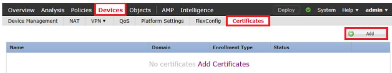
2. Select the device and the certificate is added to in the **Device\*** dropdown. Then click the green + symbol as shown in the image.
