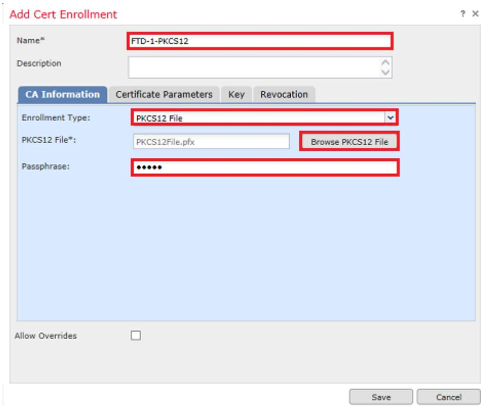
4. (Optional) The **Certificate Parameters** and **Key** tabs are grayed out as these are already created with the PKCS12, however, the **Revocation** tab to enable CRL and/or OCSP revocation checking can be modified. By default, neither are checked as shown in the image.
