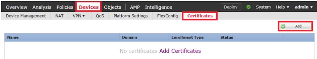
2. Select the device the certificate is added to in the **Device\*** dropdown then click the green + symbol as shown in the image.
