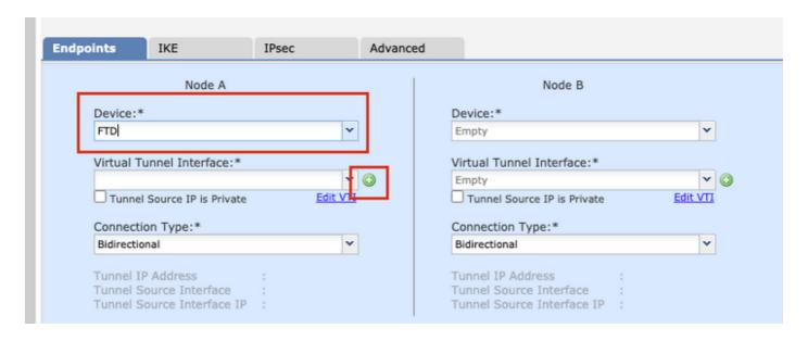
Step 5. Define the parameters of the **New Virtual Tunnel Interface**. Click **Ok**.
