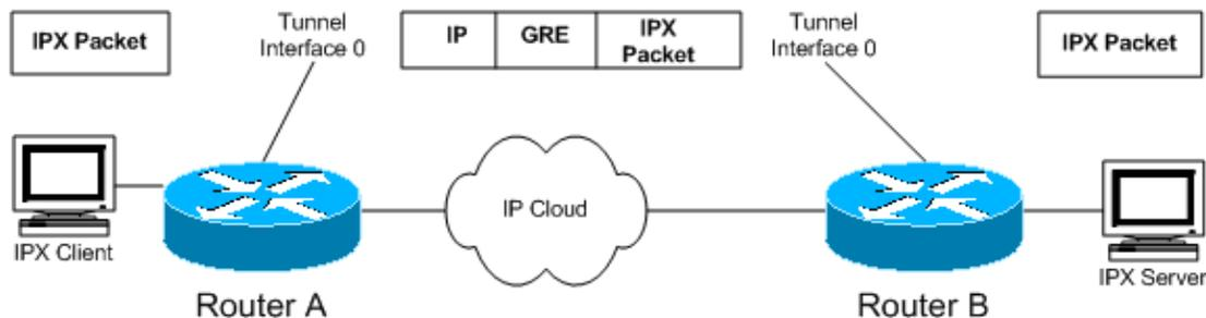
As illustrated in the diagram, GRE tunneling can also be used to encapsulate non-IP traffic into IP and send it over the Internet or IP network. The Internet Packet Exchange (IPX) and AppleTalk protocols are examples of non-IP traffic. For information on configuring GRE, see "Configuring a GRE Tunnel Interface" in [Configuring GRE](#).
