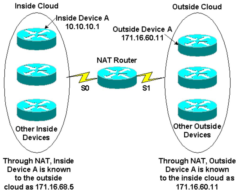
NAT is generally used to conserve IP addresses routable on the Internet, which are expensive and limited in number. NAT also provides security by hiding the inside network from the Internet.
