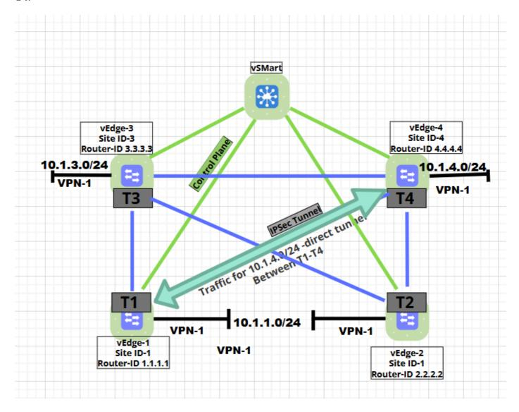
In order to provide fault tolerance and network resilience, the Control policy is configured to reroute traffic through a different path (via the specified TLOC).
