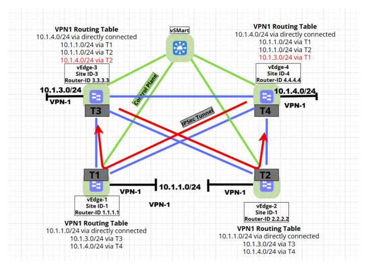
If there is a network failure that results in connectivity loss between vEdge2 and vEdge4, while the overlay tunnel between T2-T4 is down, vEdge3 still has a valid route for 10.1.4.0 via T2. Hence it sends traffic to vEdge2. vEdge2 does not have a valid Tunnel with vEdge4, so routes will no longer be active on it therefore dropping the traffic.
