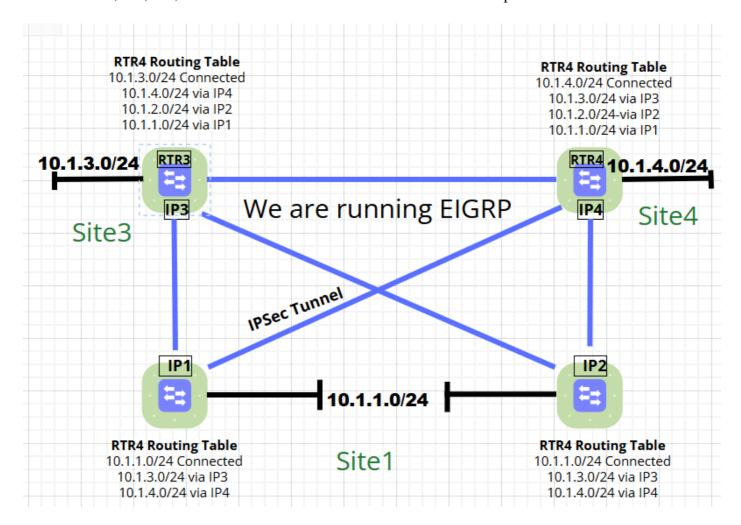
The network must be broken down, with a focus on RTR3 and RTR4 for now. On RTR3, the route to reach the 10.1.4.0/24 is via a direct tunnel between RTR3-RTR4. If the tunnel goes down, how does EIGRP react in this case? As soon as the tunnel goes down, EIGRP will run and send a query to neighboring routers for the 10.1.4.0/24 network, and based on replies received, it examines it and installs the new path for the destination in the routing table post the best path calculation.
