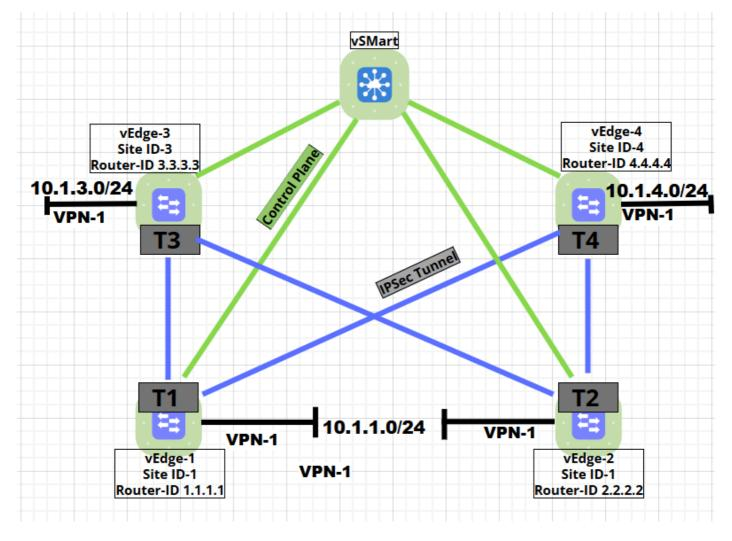
Assume that everything is set to default on the Catalyst SD-WAN Controller. The vEdge devices share the routing information directly with the Catalyst SD-WAN Controller, and the controller shares it with all vEdge devices. The next topology shows the routing table for all routers:
