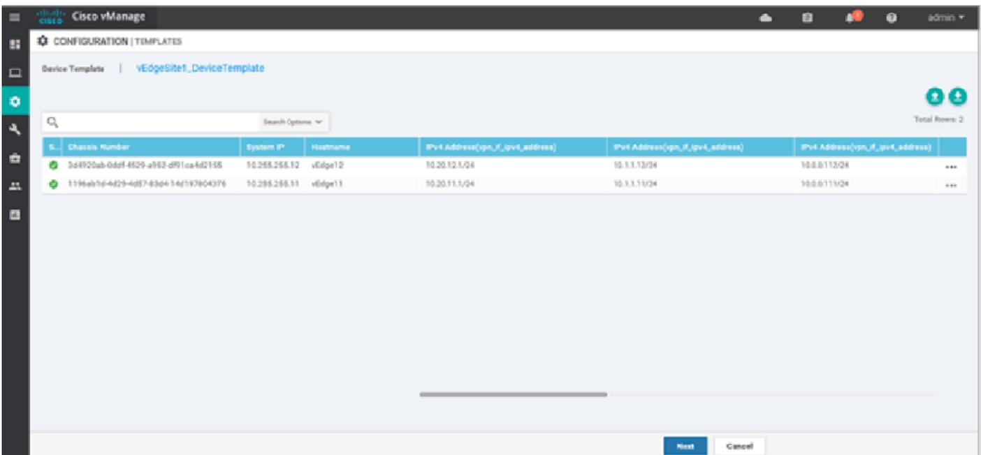
Click **Configure Devices** and confirm the configuration changes. Monitor the deployment status. The configuration is pushed to vEdge11 and vEdge12.
