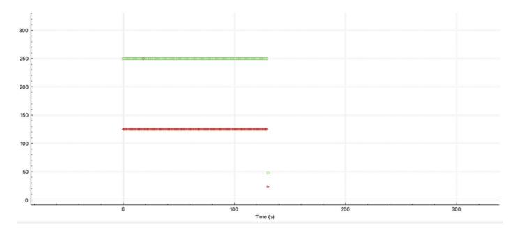
We can see the behavior with different packet size, CEM0/1/9 sends twice as much packets as CEM0/1/8, which is configured for 128 bytes.
