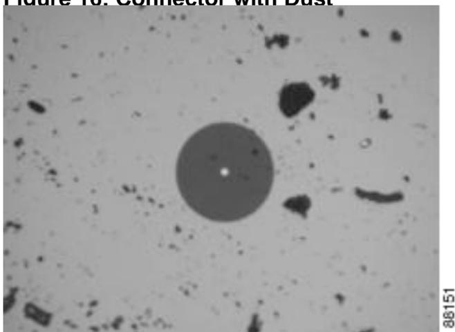
Figure 16 shows a connector with dust particles spread across the surface of the endface that needs cleaning.
