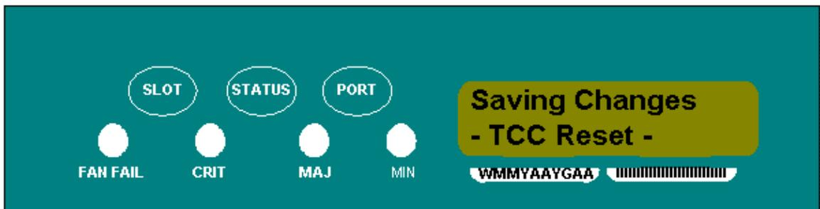
When you save a new configuration, the TCC cards reboot. The **Saving Changes** LCD appears for several minutes while the TCC cards reboot. When the LCD screen returns to the normal alternating display mode, the procedure is complete.
