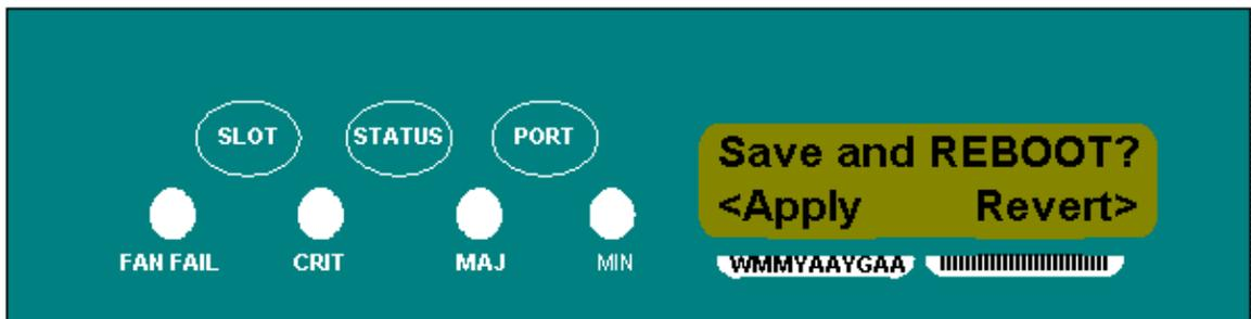
9. Press the **Slot (Apply)** button to save the new IP address configuration.
