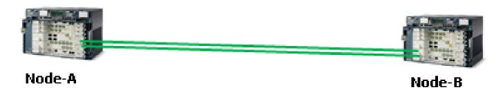
These two nodes shown in the image are typical DWDM nodes; they are connected with each other with the use of two optical fiber strands. For their management, these nodes use the OSC.
