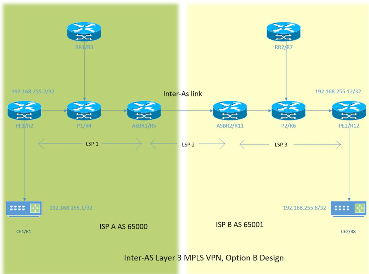
The addressing scheme is very simple. Every router has loopback1 interface described as 192.168.255.X where is X=1 when router 1 is under concern. The interface addressing is of the type 192.168.XY.X . Suppose R1 and R2 are in under consideration, configuration of the interface under the router R1 is 192.168.12.1 (here X =1 , Y = 2).
