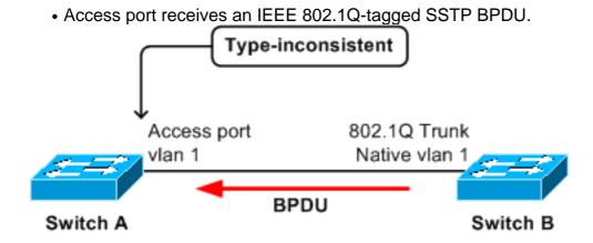
In this scenario, access port on bridge A receives, from bridge B, a tagged PVST+ BPDU from
