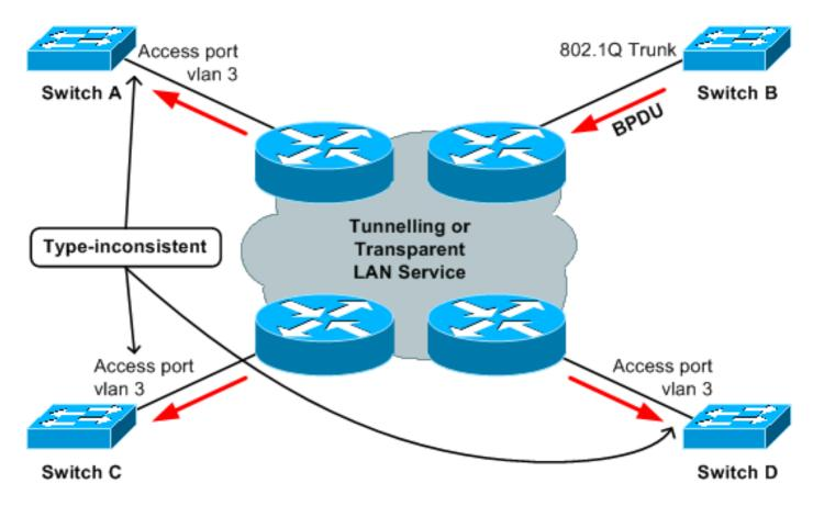
In this example, switch B is misconfigured and injects an SSTP BPDU into the cloud. This causes the ports on switches A, C, and D to become type-inconsistent. The issue is that the device that originates the "offending" BPDU is not directly connected to the affected switches. Thus, with many devices on the trunk, it can consume time to troubleshoot all of them.
