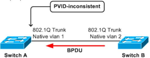
In this scenario, the trunk port on A receives a PVST+ BPDU from STP of VLAN 2 with a tag of VLAN 2. This triggers the port on A to be blocked in both VLAN 1 and VLAN 2.
