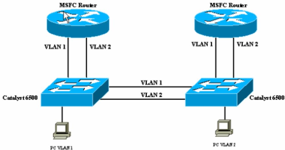
Once the Multilayer Switch Feature Cards (MSFCs) in both Catalyst 6500 are configured for bridging with the IEEE STP, both VLAN 1 and VLAN 2 are bridged together in order to form one single instance of STP. This single instance of STP contains only one STP root. Another way to view the network with the MSFC's bridging is to consider the MSFCs as separate bridges. One instance of STP that involves the MSFCs can result in an undesirable network topology.
