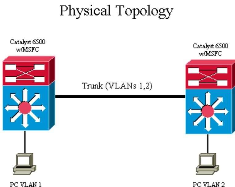
The diagram shown illustrates a physical topology of a typical Layer 3 (L3) network.
