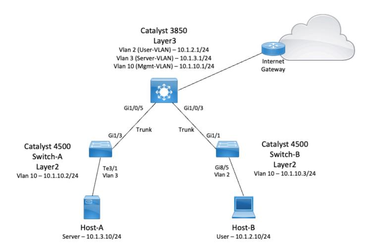
In this diagram, the Catalyst 3850 switch provides the Inter-VLAN routing function between the different VLANs. The Catalyst 3850 switch can act as an L2 device with the disablement of IP routing.
