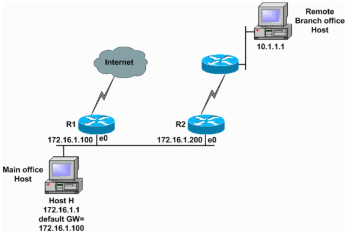
This debug message shows router R1, as in the network diagram, sending an ICMP redirect message to Host H (172.16.1.1).
