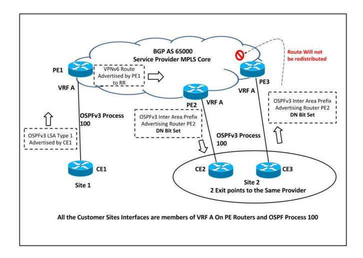
Based on the network topology, PE2 sets the DN Bit for the redistributed LSA and this LSA is never considered for route calculation in OSPF Process 100 on PE3. So PE3 never redistributes this route back into MP-BGP.
