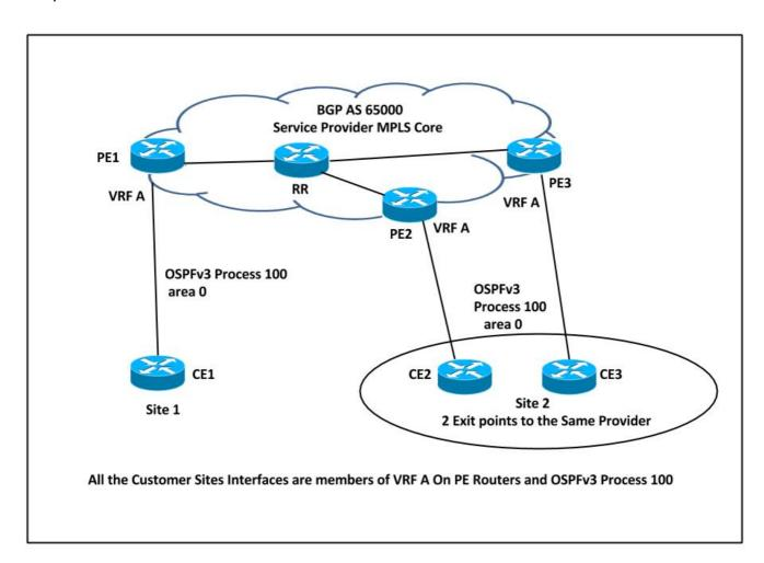
In this setup, there is a possibility of a loop. For example, if CE1 advertises the OSPFv3 LSA Type 1 to PE1, which redistributes the route into VPNv6 and advertises it to PE2, then PE2 in turn advertises the Inter-Area-Prefix LSA to CE2.
