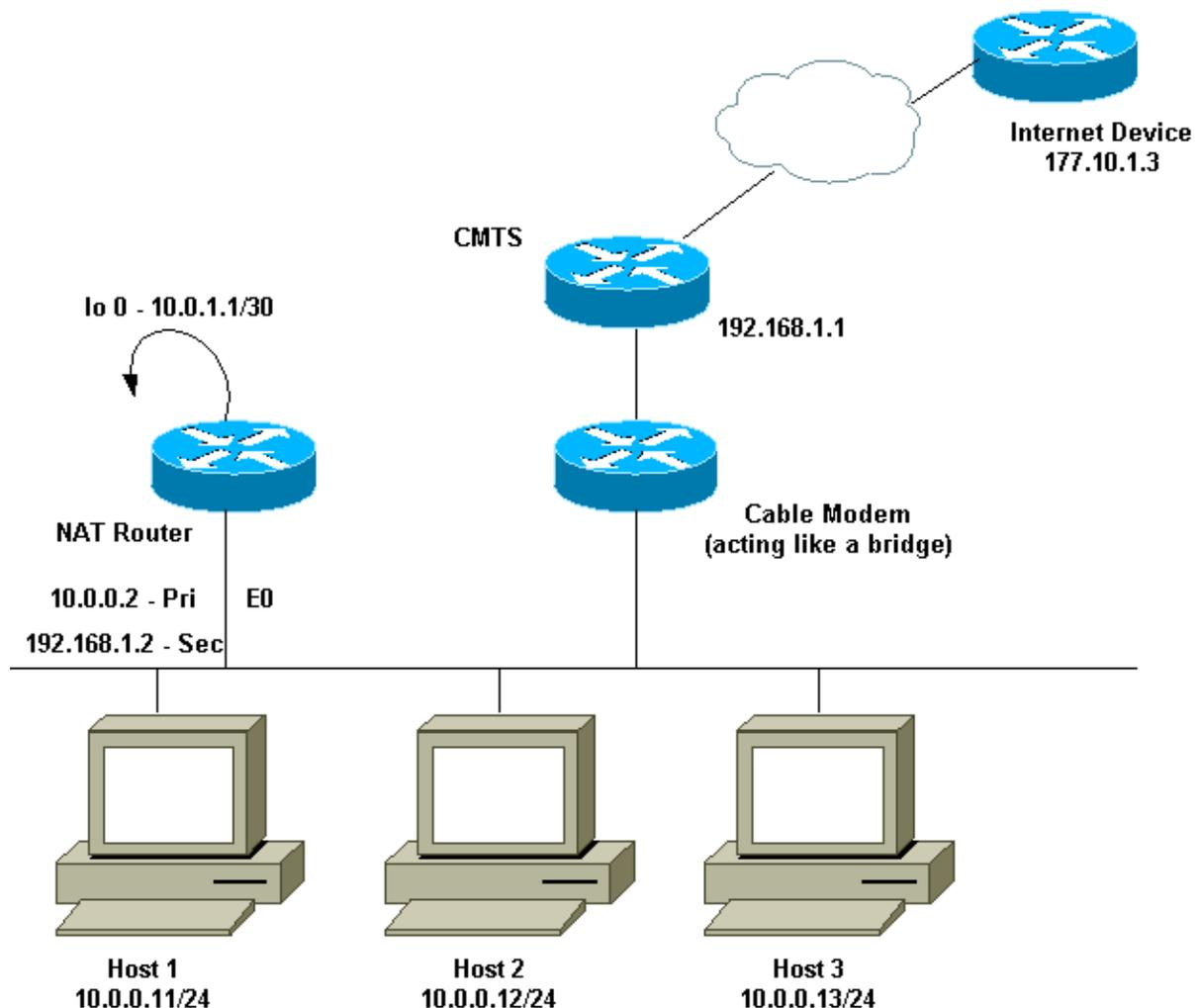
The above network diagram is very common in a cable modem set up. The Cable Modem Termination System (CMTS) is a router and the Cable Modem (CM) is a device that acts like a bridge. The problem we face is that
