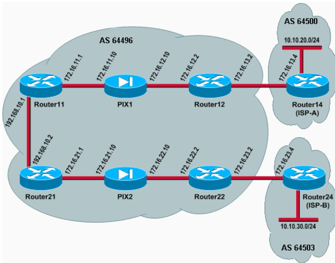
In this network setup, Router12 and Router22 (which belong to AS 64496) are multihomed to Router14 (ISP-A) and Router24 (ISP-B) respectively, for redundancy. The internal network 192.168.10.0/24 is on the inside of the firewall. Router11 and Router21 connect to Router12 and Router22 through the firewall. PIX1
