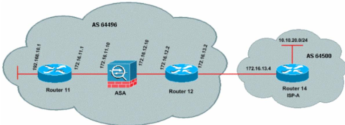
PIX/ASA version 7.x and later introduces an additional challenge when you try to establish a BGP peering session with MD5 authentication. By default, PIX/ASA version 7.x and later rewrites any TCP MD5 option included on a TCP datagram that goes through the device and replaces the option kind, size and value with NOP option bytes. This effectively breaks BGP MD5 authentication, and results in error messages like this on each peering router:
