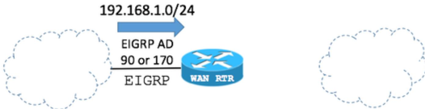
The key point is that BGP can advertise or redistribute EIGRP routes (with the help of the next Router configuration). If that is the case, the EIGRP route is now added to the BGP table.
