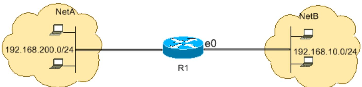
This configuration allows the IP packets with an IP header that has a source address in the network 192.168.10.0/24 and a destination address in the network 192.168.200.0/24 access to NetA. There is the implicit deny all clause at the end of the ACL which denies all other traffic passage through Ethernet 0
