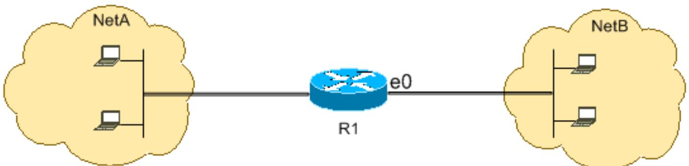
This configuration permits TCP traffic with destination port values that match WWW (port 80), Telnet (port 23), SMTP (port 25), POP3 (port 110), FTP (port 21), or FTP data (port 20). Notice an implicit deny all clause at the end of an ACL denies all other traffic, which does not match the permit clauses.
