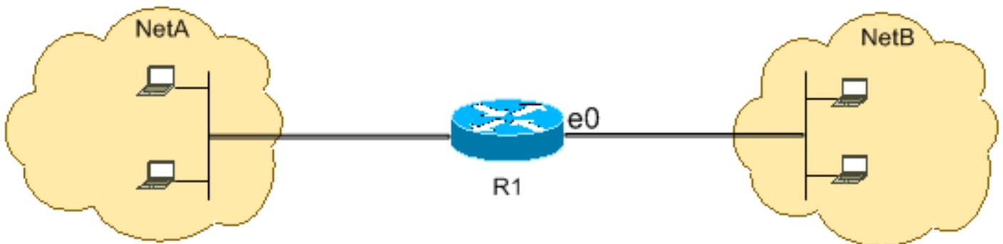
Telnet uses TCP, port 23. This configuration shows that all TCP traffic destined to NetA for port 23 is blocked, and all other IP traffic is permitted.
