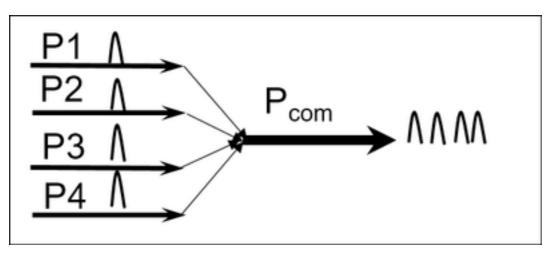
When each channel has different power at input then the Composite Power formula looks like this:
