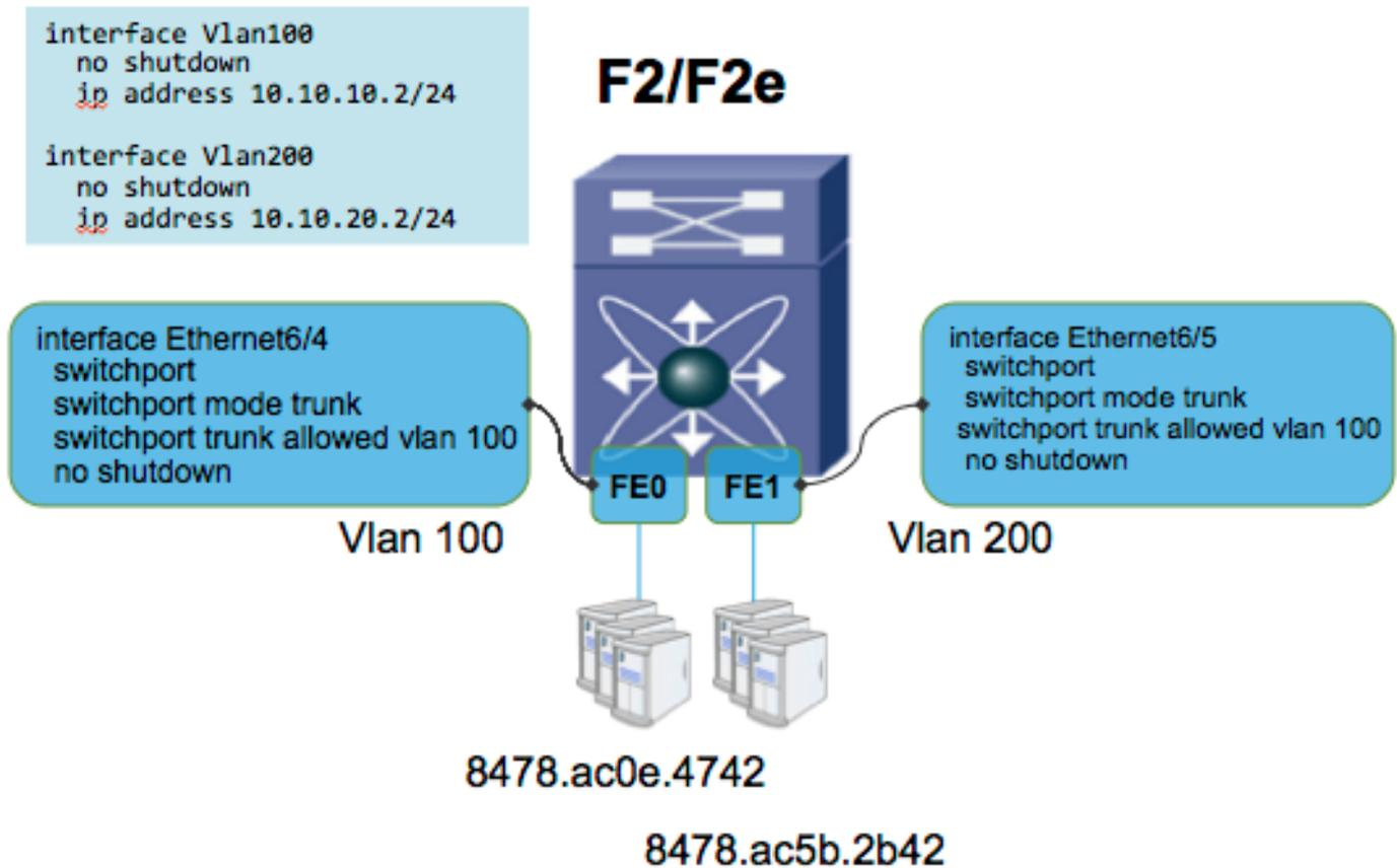
The MAC table will look like this, where MAC address is synced between FEs even though the vlan is pruned. This is because Switch Virtual Interface (SVI) is enabled which requires the FE to know about MAC addresses from other vlans as well.
