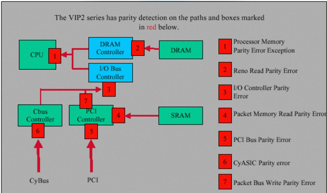
As shown in this diagram, there are seven different types of parity errors that can occur on a VIP. Note that errors can be received from another source and might not have originated within the VIP itself. The source of the parity error can be from the Route/Switch Processor (RSP), another VIP, or from poorly seated or faulty port adapters. In order to properly understand a VIP crash, it is important to diagnose the source of the crash.
