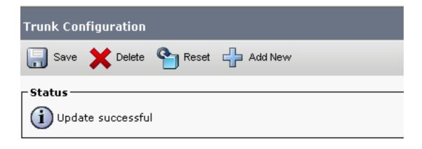
The configuration changes will not take effect on the trunk until a reset is performed. Use the Reset button or Job Scheduler to execute the reset.
