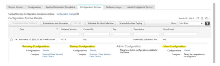
If blocking TFTP between the 9800 WLC, and the Prime server. The configuration archive will fail as TFTP is the used protocol between the WLC and the server.
