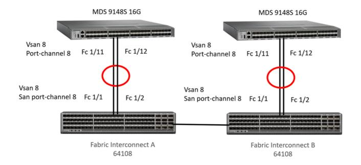
This example shows san port channel configuration between FI managed by Intersight and MDS. Used fc1/1 and fc1/2 interfaces for Fabric Interconnect and fc1/11 and fc1/12 for MDS.
