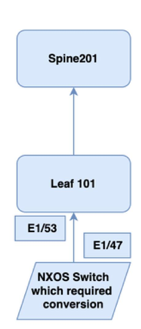
Add the appropriate Node 101 (Existing ACI switch) and interface E1/53 on Leaf 101 to be used for POAP (Only Fabric Links can be used for POAP on Leaf/Spine).
