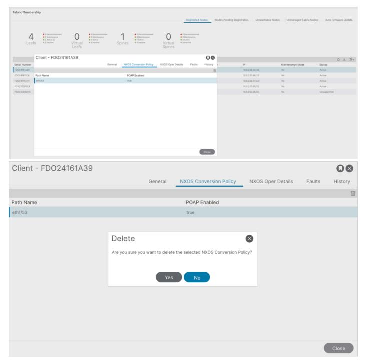
++ You also encounter an Fault F427 when you configure POAP, please ensure that fault is cleared post s This fault is an reminder that you have configured an port on ACI Leaf switch for POAP usage
