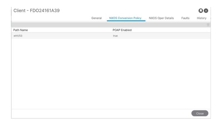
**Step5:** Connect Nexus node to the Leaf 101 interface E1/53 then you are going to see the new switch node under Nodes Pending registration. In this example we are using port E1/47 on new NXOS switch.
