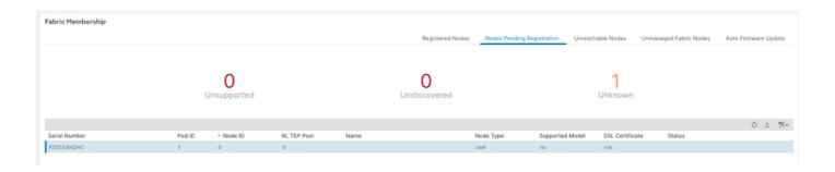
**Step6:** Register the new switch node, right click and select register.
