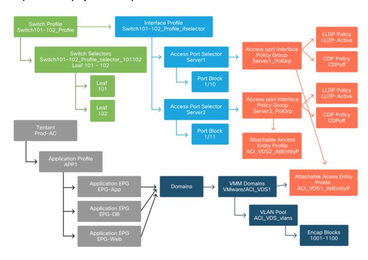
If Pre-provision was set for an EPG in the ACI\_VDS1 VMM Domain, then VLANs would be deployed on links for Server1 but not Server2 as Server2's AEP does not include the ACI\_VDS1 VMM Domain.
