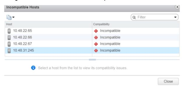
So, when creating a VMM Domain make sure to select the correct 'DVS Version' such that the necessary ESXi servers can be added to the DVS.
