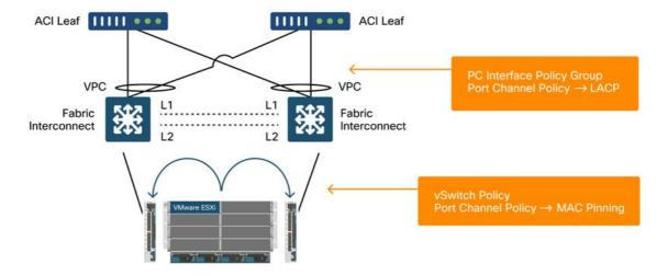
When MAC Pinning is configured on the Port-Channel Policy as part of the vSwitch Policy in ACI, this will show as 'Route based on the originating virtual port' teaming configuration of the port groups on the VDS.
