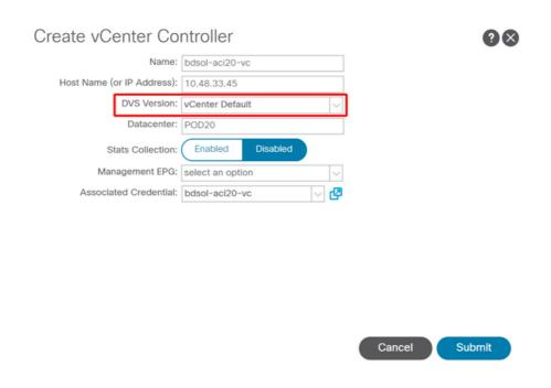
This means that in the example of a vCenter running 6.5 and ESXi servers running 6.0, the APIC will create a DVS with version 6.5 and hence the vCenter administrator will be unable to add the ESXi servers running 6.0 into the ACI DVS.
