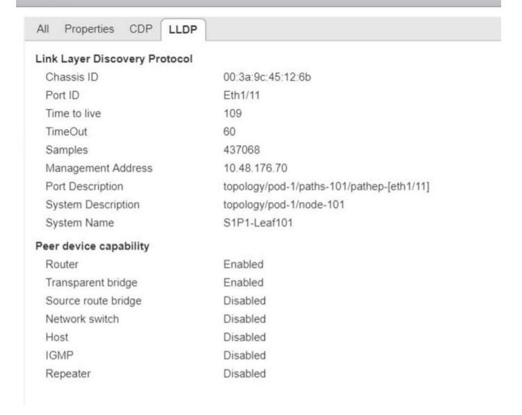
If the leaf LLDP adjacency cannot be seen from the ESXi host, this is often caused by using a network adapter which is configured to generate LLDPDUs instead of the ESXi OS. Make sure to validate if the network adapter has LLDP enabled and hence is consuming all LLDP information. If this is the case, be sure to disable LLDP on the adapter itself so it is controlled through the vSwitch policy.
