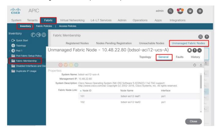
With LLDP or CDP discovery in place, ACI can determine the topology for such LooseNodes, given that the hypervisor downstream of the intermediate switch is managed through VMM integration, and the leaf itself has an adjacency to the intermediate switch from downstream.
