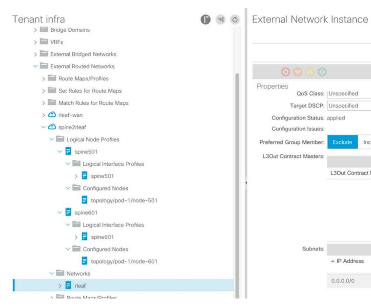
Now that you've configured OSPF L3Out from Spine (node-501 & node-601) to the IPN device. The OSPF adjacency should be up and routes are exchanged provided the OSPF on the IPN is configured correctly. So, check the OSPF neighbourship from Spine to IPN device.
