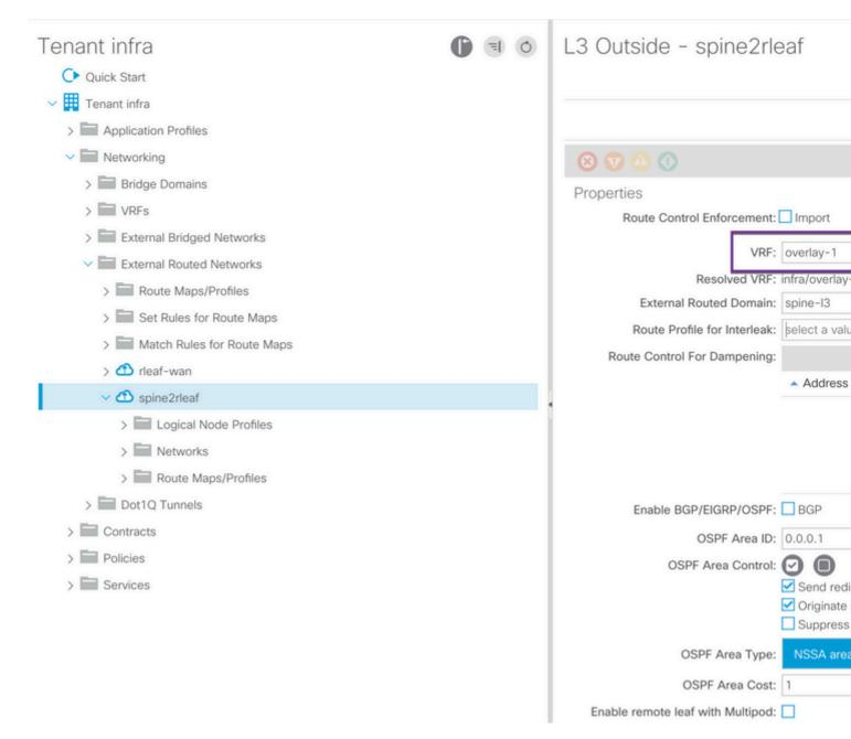
Configure the Node profile for each spine (in this example node-501 & node-601) connected to IPN. The example for node-501 is shown here. Follow the same steps for node-601. Image snippets may show different IP addressing schemes.
