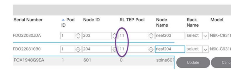
**Note**: Ensure to select the correct **RL TEP Pool** you configured in Step 1. Also, check and confirm the **Role** is selected as a remote leaf automatically when you select the **RL TEP POOL** from the dropdown.
