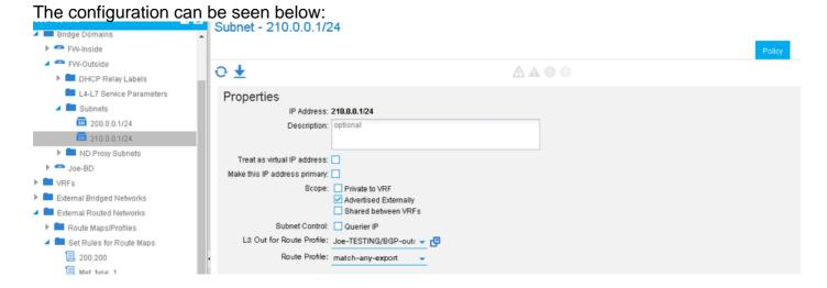
The only difference between applying the route-profile at the BD level vs. the BD subnet level is
