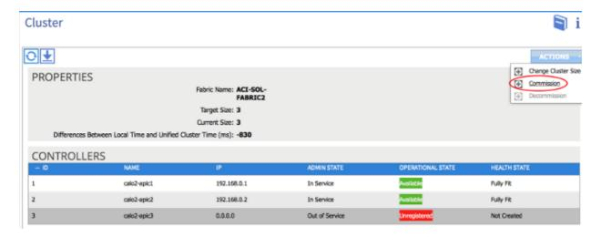
The APIC receives an IP address, which is reflected in the web interface of the APIC.
