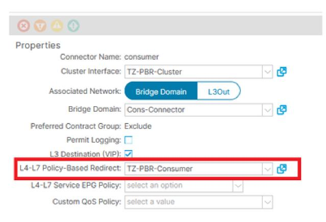
F0759: graph-rendering-failure - "Service graph for **tenant** < **tenant** > could not be instantiated. Function **node** < **node** > configuration is invalid."
