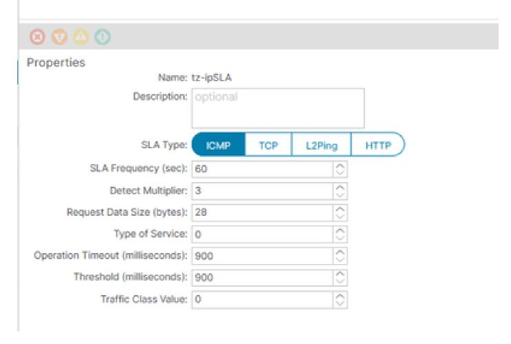
The IP SLA policy has to be mapped to the PBR-node IP by means of a Health Group.
