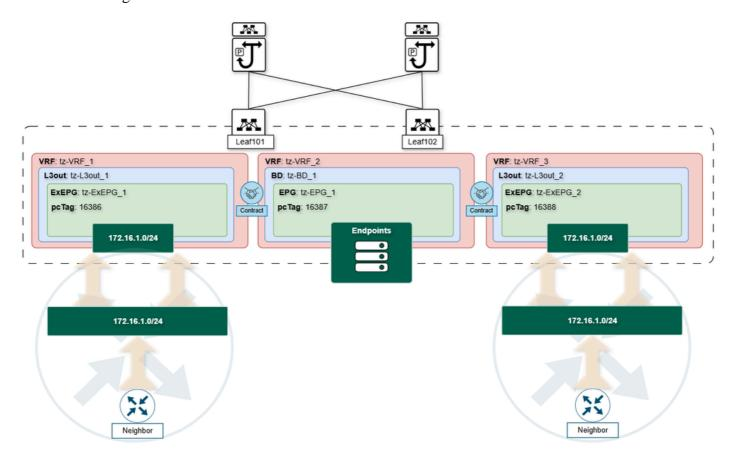
• Local-to-VRF L3Out ExEPG Overlapping with Leaked Subnets: In designs where route leaking is used, if a local L3Out ExEPG is configured with the same subnet as a leaked subnet, the local routing entry always take precedence over the leaked routes.
