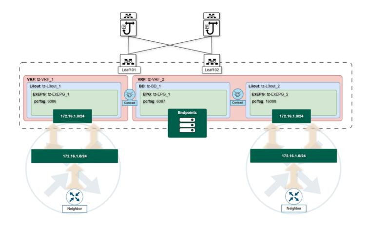
These situations highlight that the asymmetric forwarding issues arise from the classification and forwarding decision layer, not from the routing table itself. While subnet classification associates a subnet with a specific L3Out and ExEPG for policy enforcement, the routing table can point to a different L3Out destination. This mismatch can cause traffic to be forwarded inconsistently, leading to potential connectivity problems or policy enforcement gaps.
