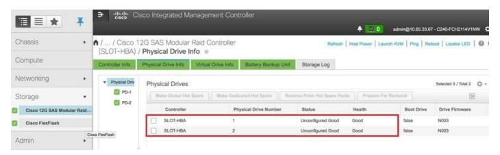
Create a virtual drive from the physical drives with RAID Level 1:
