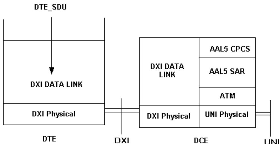
The important part about this setup is that an ADSU is required to convert from frames into ATM cells. Manufacturers of standard DSU/CSUs also offer special ADSUs. Contact your telco provider for recommended ADSUs. Kentrox [is](#) one manufacturer of ADSUs.
